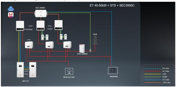
Mixed inverters in parallel, on/off grid working, BACK-UP in parallel(SEC3000C)
