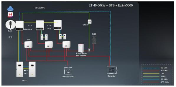
On/off grid working, BACK-UP in parallel(SEC3000C, up to 10)
