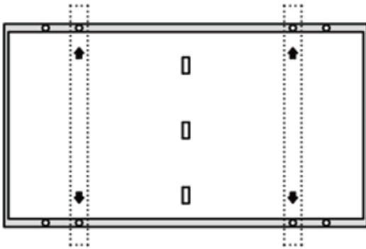
The long frame uses the inner four holes (990mm) for bolt installation
