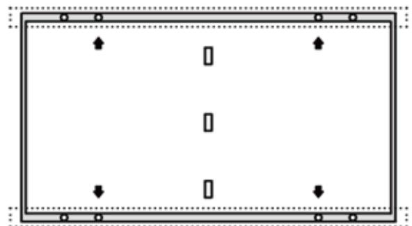
The long frame uses the inner four holes (990mm) for bolt installation
