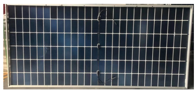
Sample 3#: Burning brand test (back)
