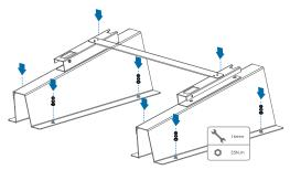
**Step 5** Uplift the inverter, and fix it onto the rack by anchoring two supplied M6\*65 bolts on both sides.
