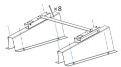
**Step 4** Drill holes according to the marks and fix the rack.
