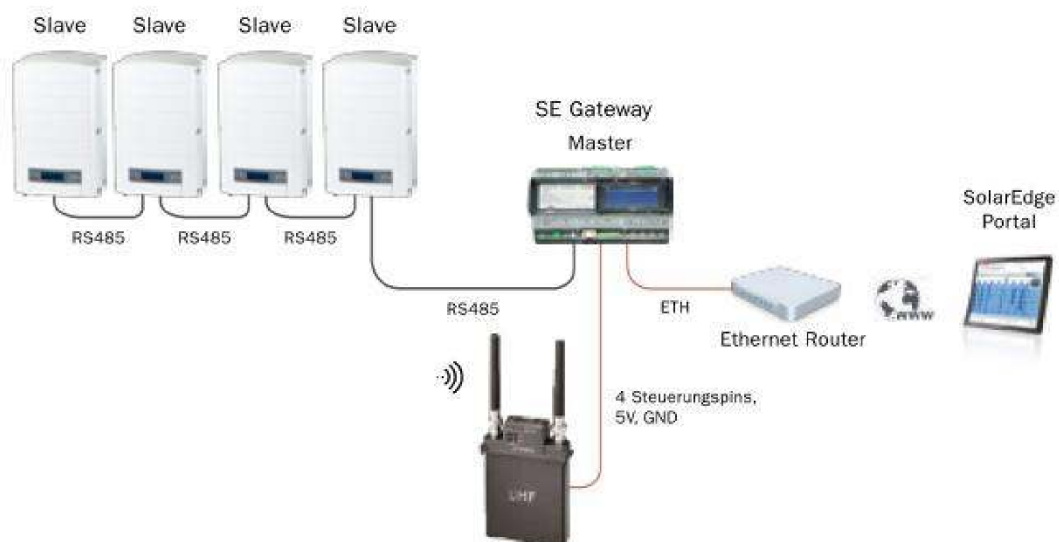
Figure 3 – Scheme of an installation
