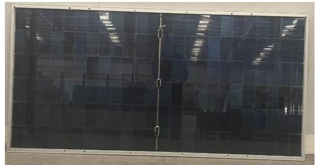
Sample 2#: Spread of flame test (back)
